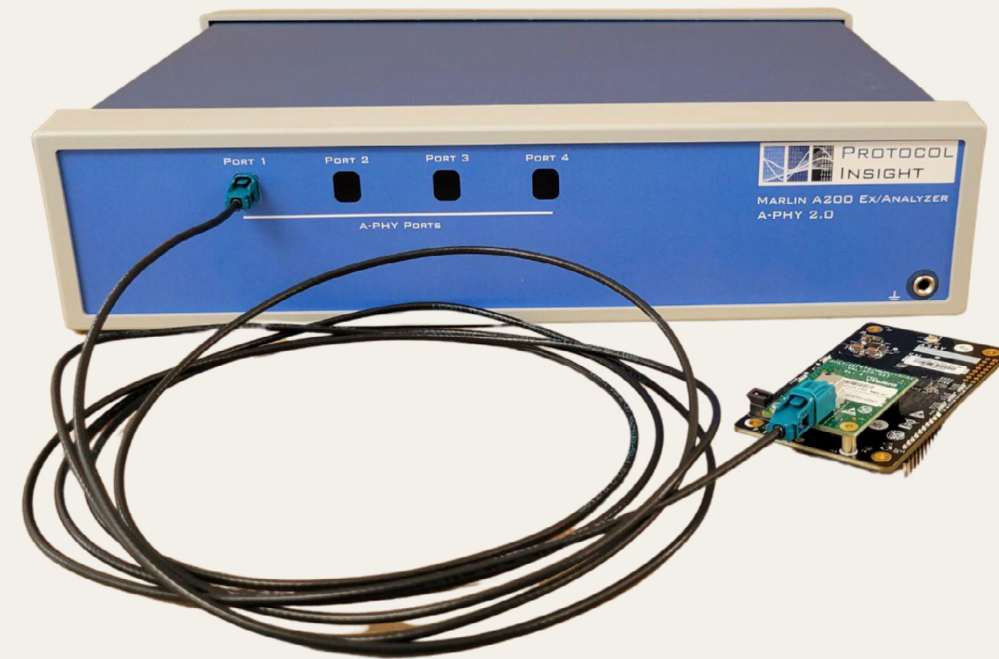
Protocol Insight's Marlin A200 protocol analyzer and exerciser
